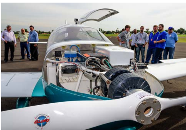
Sora-e is equipped with two Enrax thrusters, manufactured in Slovenia.
